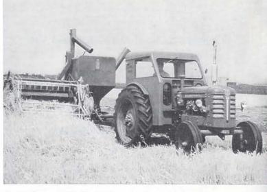
The BM-Volvo 350 has Terra-Trol hydraulics, giving most regular working depth regardless of surface conditions and type of soil. The Terra-Trol also ensures automatically that maximum implement weight is transferred to the driving wheels. The great lugging power of the engine in the 350 enables it to overcome the toughest obstacles. Big rear wheels and differential lock very effectively reduce slipping.
