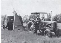
The BM-Volvo 350 has a transmission offering 10 forward speeds and 2 reverse, meaning that the right speed can be selected for virtually every job. Independent p.t.o., high p.t.o. ratings and judiciously selected engine speeds at the right p.t.o. speed make the 350 particularly suitable for p.t.o. powered machinery.
