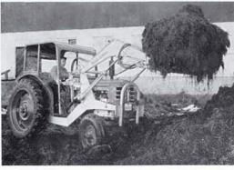
The BM-Volvo 350 has been designed for use as a front loader. The front axle is of heavy-duty type and the wheels are large. Suitable attachment points are provided on the frame. The 350 has a fully independent hydraulic system – the loader gear functions even when the clutch is disengaged and gears are changed.
